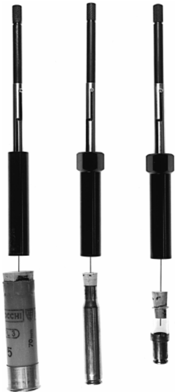
FIG. 1—SPME sampling from a shotgun shell, from a sporting rifle cartridge and from a pistol cartridge. The pistol cartridge was too short for direct insertion of the SPME fiber and was therefore prolonged with a plastic tubing. The sampling time was 20 min in all experiments.
